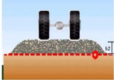
Aggregate and subgrade interaction (a) without geosynthetic layer and (b) with geosynthetic layer
